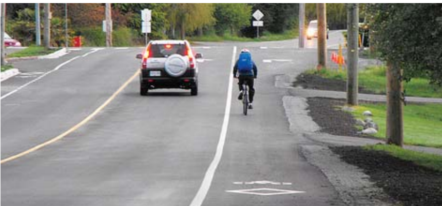
Figure 3.4-10 Bicycle and Pedestrian Shared Shoulder
